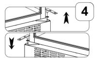
5. Locate the glass door to the designated position making sure that the door shaft enters the door hole at the left upper corner of the glass door. Install the two screws that are used to connect the left lower hinge with the glass door and tighten them before the door is leveled. Then remove the handle from the left side and install it on the right side of the glass door.
